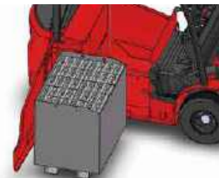
Battery side removed by forks (Opt.)
