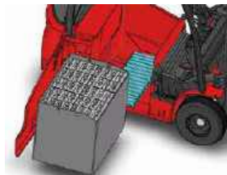
Battery side roll out by roller (Opt.)
